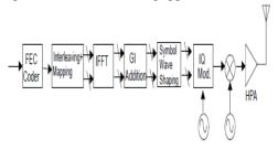
Fig. 3 WLAN (802.11a) transmitter [5]
